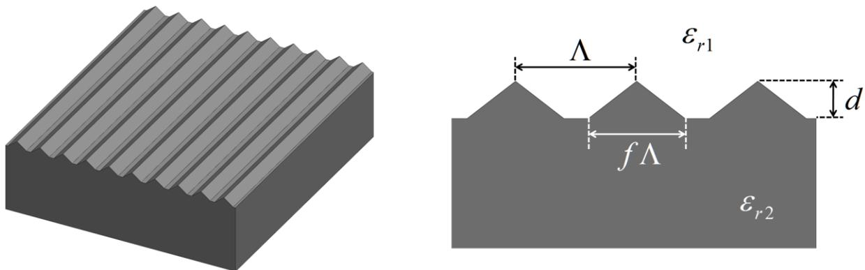
**Figure 1. Diffraction grating with infinite substrate**
