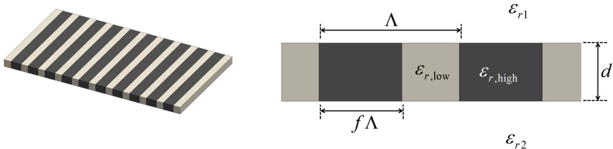
**Figure 2. Diffraction grating in air**
